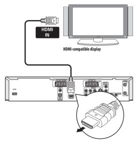
• The arrow on the cable connector body should be face up for correct alignment with the connector on the recorder.
